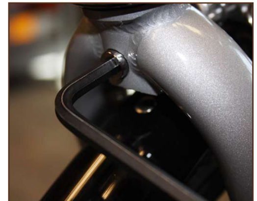
Fig. 4: Front fender L-bracket installation (for road brakes)
