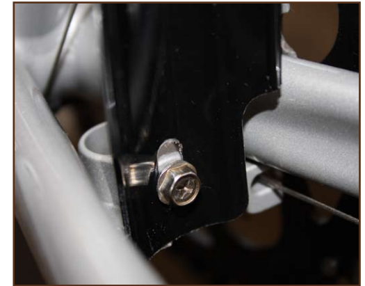
Fig. 10: Rear fender to chainstay bridge attachment
