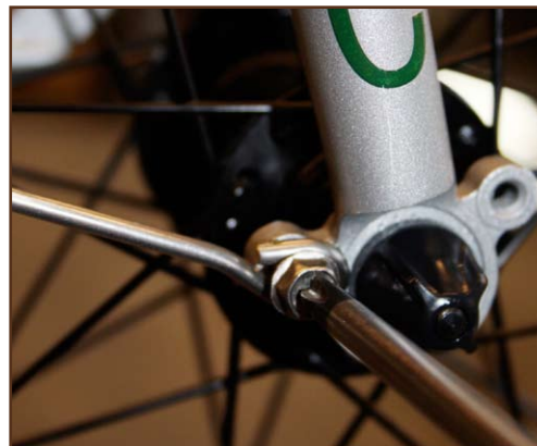
Fig. 5: Front fender stay attachment
