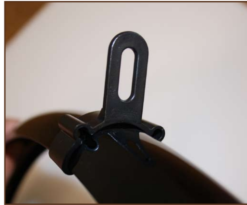
Fig. 7: Rear fender clip
