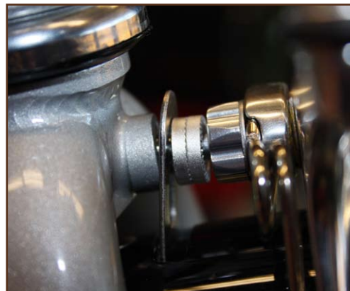
Fig. 3: Front fender L-bracket installation (for road brakes)
