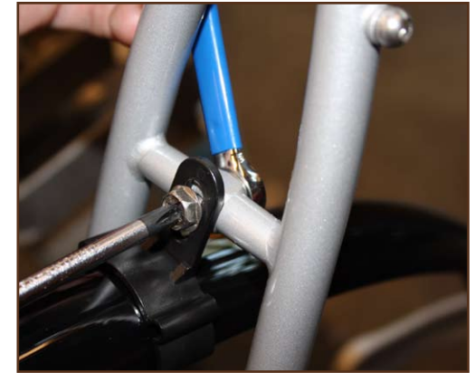
Fig. 8: Rear fender clip installation
