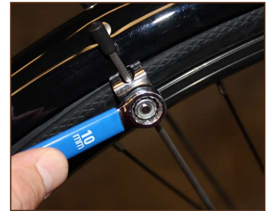
Fig. 12: Rear fender stay adjustment
