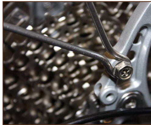
Fig. 11: Rear fender stay attachment
