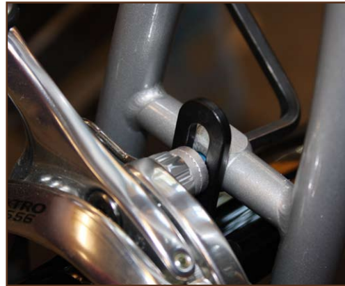
Fig. 9: Rear fender clip installation (for road bikes)
