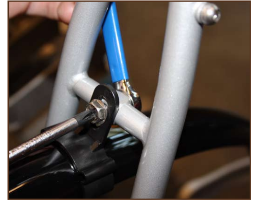
Fig. 8: Rear fender clip installation
