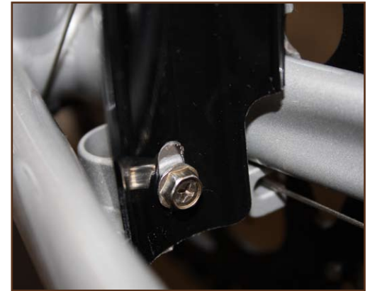
Fig. 10: Rear fender to chainstay bridge attachment
