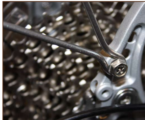
Fig. 11: Rear fender stay attachment
