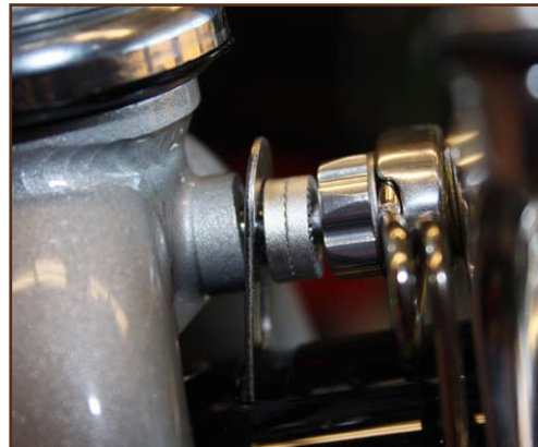
Fig. 3: Front fender L-bracket installation (for road brakes)
