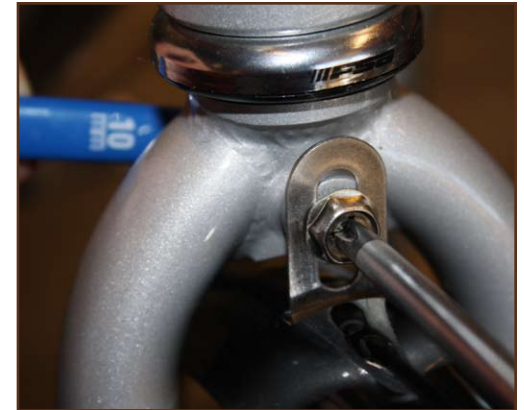
Fig. 2: Front fender L-bracket installation
